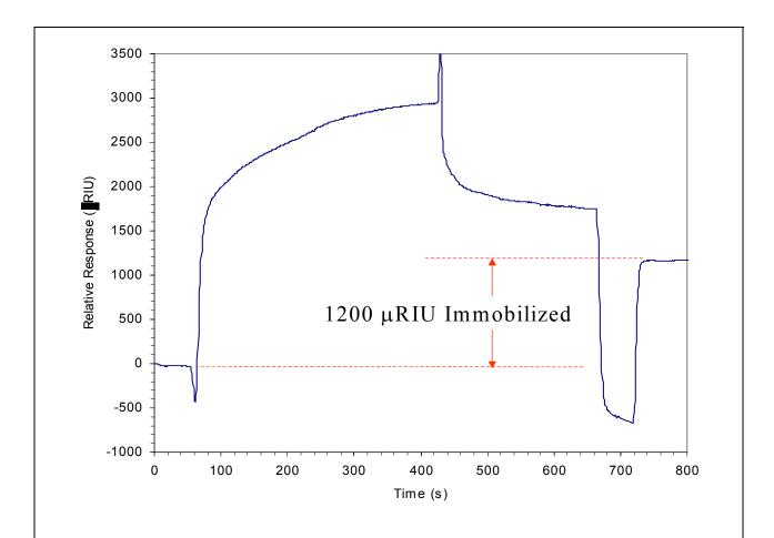
Figure 1. Injection of reduced goat IgG over an SPDP treated protein coated surface. The reduced antibody is linked to the surface by displacing pyridyl groups via disulfide exchange. An acid wash removed weakly adsorbed material leaving 1200  $\mu$ RIU of antibody immobilized.
