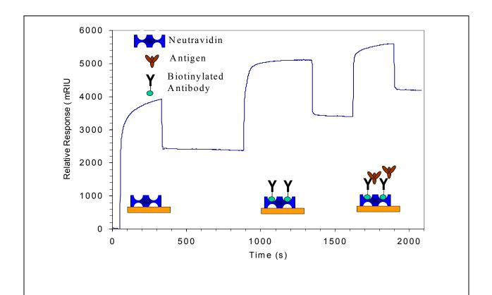
Figure 2. Direct immobilization of neutravidin (2400  $\mu$ RIU) to gold surface followed by affinity capture of biotinylated antibody (1000  $\mu$ RIU). The third injection is antigen (800  $\mu$ RIU), and is used to confirm the binding activity of the immobilized antibody.
